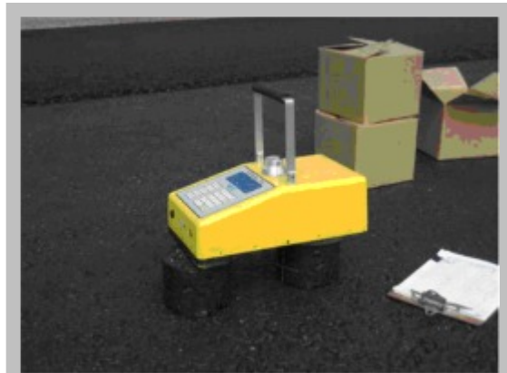
This PaveTracker density gauge, shown measuring asphalt samples, operates effectively without radioactive materials.
