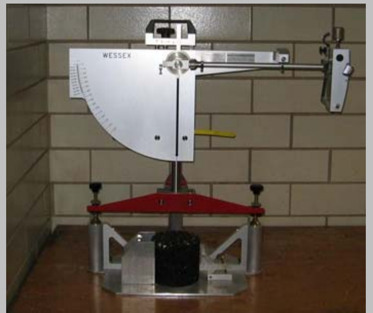
The British Pendulum helps determine a pavement's mean texture depth, a factor in modeling friction and noise. (Image courtesy of UW–Madison Modified Asphalt Research Center)
